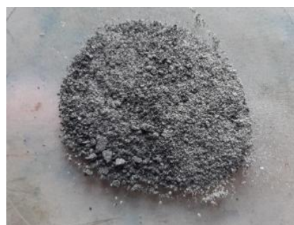
Fig. 10 ECR treated aluminum hydroxide sludge from dyes after drying
